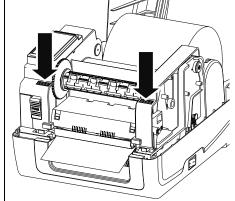
(6) Close the print head mechanism by both hands and make sure the latches are engaged securely.
