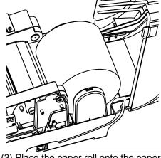
3) Place the paper roll onto the paper roll mount. (If your paper width is 4 inch, you can remove the fixing tabs from the supply spindle.)
