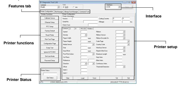
(3) The detail functions in the Printer Function Group are listed as below.
