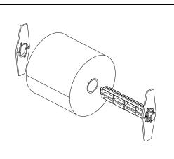
(2) Insert the media supply spindle into the paper roll and use two fixing tabs to fix the paper roll onto the center of the spindle.
