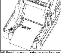
(5) Feed the paper, printing side face up, through the media bar, media sensor and place the label leading edge onto the platen roller. Move the media guides to fit the label width.
