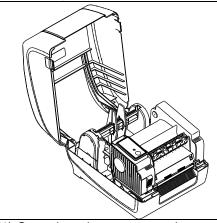
Open the printer top cover by pressing the top cover open tabs located on each side of the printer.
