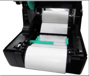
1. Refer to chapter 3.3.1 to install the label. Use "Diagnostic Tool" to set the media sensor type and calibrate the selected sensor.
