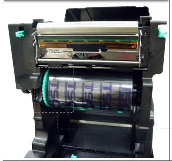
6. Insert the left side of ribbon supply spindle to the ribbon supply hub first then insert the right side of ribbon supply spindle to the hole at the right side of ribbon mechanism.
