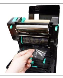
7. Pull the leader of the ribbon through the print head and stick the leader of the ribbon onto the ribbon rewind paper core.
