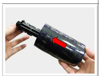
5. Insert the ribbon to the ribbon spindle.
