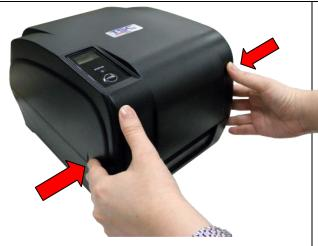
Open the printer top cover by pressing the top cover open tabs located on each side of the printer.
