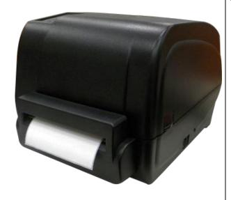
Close the print head mechanism and printer cover. Use the DiagTool to set the printer for cutter mode by selecting "CUTTER" option for Post-Print Action setting then click "Set" button to enable the cutter mode. Press the FEED button to test.
