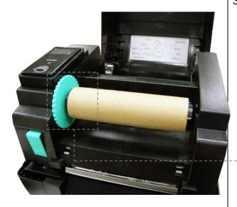
Insert the left side of ribbon rewind spindle to the ribbon rewind hub first then insert the right side of ribbon rewind spindle to the hole at the right side of ribbon mechanism.
