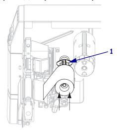
Pull the end of the ribbon under the printhead assembly (1) and out the front of the printer. Extend the ribbon approximately 24 in. (610 mm) out of the printer.
