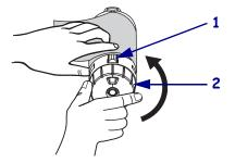
**3.** Slide the used ribbon off of the ribbon take-up spindle and discard.
