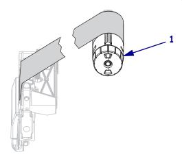
2. To loosen the ribbon, squeeze it against the ribbon take-up spindle tension blades (1). At the same time, turn the ribbon take-up spindle release knob counterclockwise (2). The tension blades collapse into the ribbon take-up spindle, loosening the ribbon.
