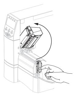
**2.** Insert the ribbon into the printer. In this step, follow the instructions for the Thermal Transfer option installed in your printer.
