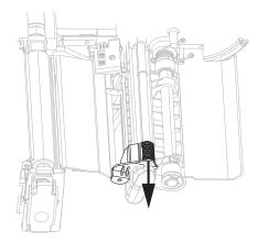
3. Insert media into the printer. Follow the instructions for roll or fanfold media, as appropriate.
