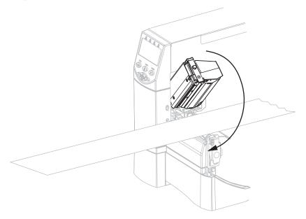
**4.** Wind the ribbon clockwise onto the ribbon take-up spindle (1).
