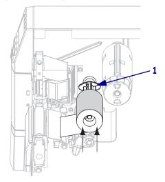
**c.** Pull the end of the ribbon under the printhead assembly (1) and out the front of the printer. Extend the ribbon approximately 24 in. (610 mm) out of the printer.
